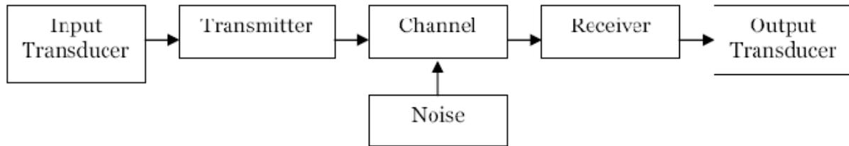
Fig. 1 Block Diagram of a Communication System
