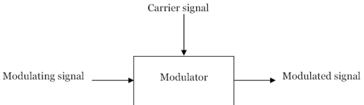
Fig. 2 Block Diagram of a Modulation Process
