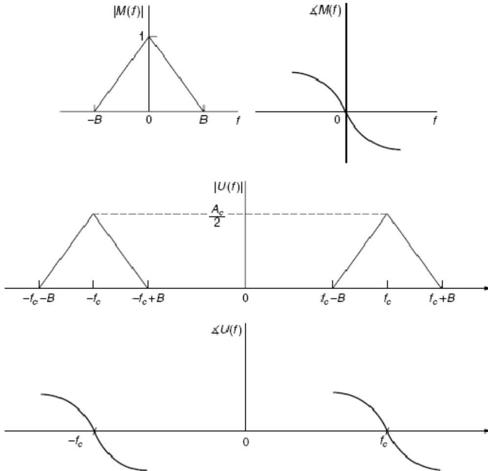
Fig.5 Magnitude and phase spectra of the message signal  $m(t)$  and the DSB AM modulated signal  $u(t)$ .
