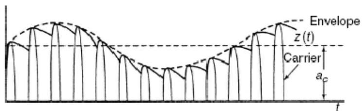
Fig.7 Envelope detection of conventional AM signal.
