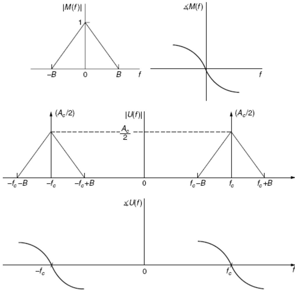
Fig.6 Magnitude and phase spectra of the message signal  $m(t)$  and the conventional AM signal.
